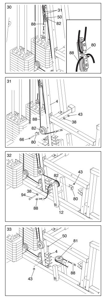
34. Route the Press Cable (88) around a 3 1/2" Pulley (82). Attach the Pulley and a Cable Trap (80) to the Press Frame (12) with a 3/8" x 3" Bolt (94), a 3/8" Washer (38) and a 3/8" Nylon Jamnut (43).
